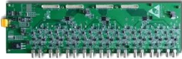
Fig. 10. (color online) Prototype of the LHAASO WCDA AFE.
