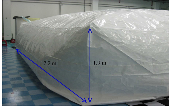
Fig. 2. One of the Tyvek bags (7.2 m in side length and 1.9 m in height) filled with air.
