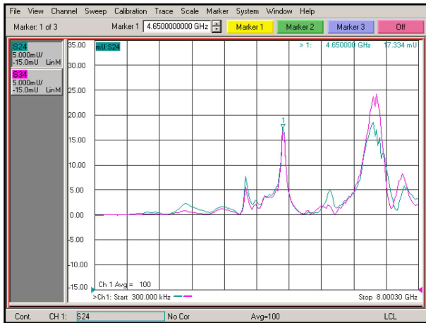
Fig. 4. (color online) S -parameter test when having strong TE modes coupling.
