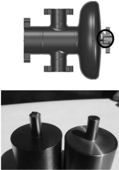
Fig. 1. The top picture is the geometry of BNL half cell 1.3 GHz plug gun. The Nb plug is located inside the circle. The bottom picture is the fabricated Nb plugs. The GaAs crystal is welded on the top of Nb plugs. The left one is of flat tip design. The right one has a recessed structure that the GaAs crystal merges into the Nb plug, which is different from the original design shown on the left. The GaAs crystal size is 2 mm × 2 mm × 0.6 mm.
