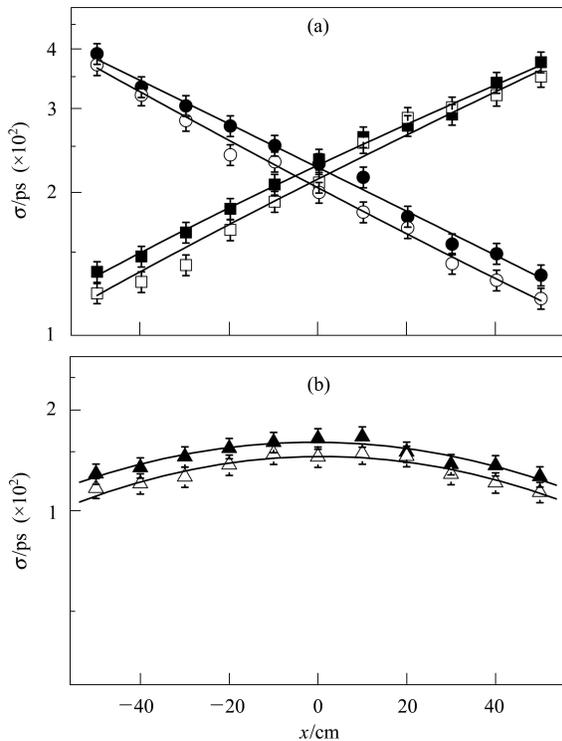
Fig. 4. Time resolutions of (a)  $\sigma_{t_l}$ ,  $\sigma_{t_r}$  and (b)  $\sigma_{t_{av}}$  versus  $x$  with two different discriminators. Solid symbols are the results for the CFD, and open symbols are the results for the LED corrected for the time walk effect.
