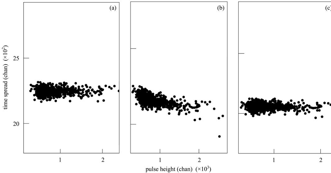
Fig. 3.  $t_1 - t_s$  signal time spread versus pulse height for  $x = 0$  (a) with the CFD; (b) with the LED without time walk effect corrections; (c) with the LED with time walk effect correction.
