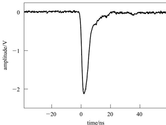
Fig. 1. A typical PMT pulse signal observed by a digital oscilloscope.
