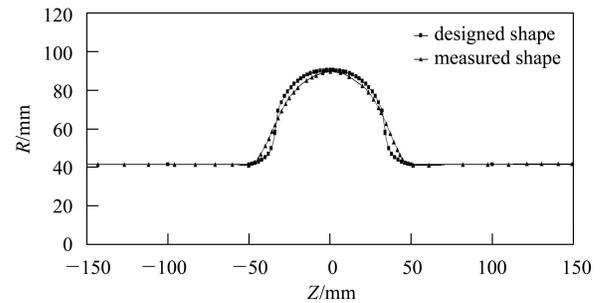
Fig. 1. Comparison between the measured shape and the designed shape for the niobium cavity.
