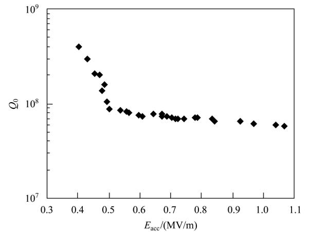
Fig. 5.  $Q_0$  versus accelerating field curve at  $4.2$  K for the niobium cavity just after ultrasonic rinsing.
