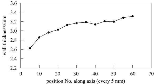
Fig. 3. The wall thickness distribution of the niobium half-cell along the axis direction after deep drawing.
