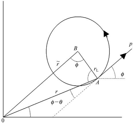
Fig. 1. Projection of the electron orbit (indicated by circle) on the cross-sectional plane.  $r_L$  is the Lamor radius. Point 0 is the centre of the waveguide and point B is the centre of the cyclotron orbit. Point A is the instantaneous position of the electron.
