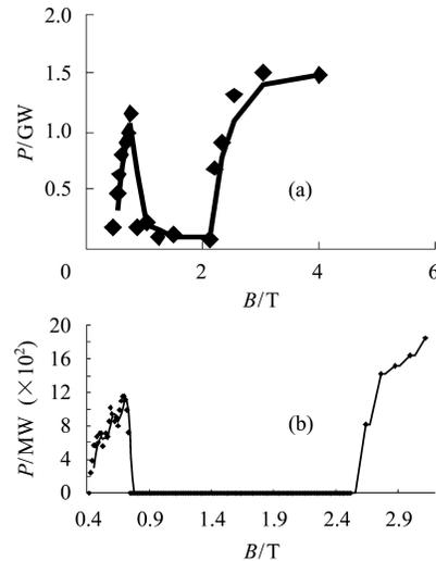
Fig. 6. The relationships between the output power and the guiding magnetic field which are through (a) simulation (b) experiment.
