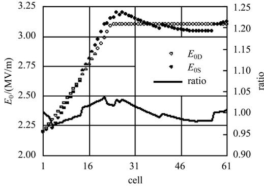
Fig. 4. The  $E_0$  distribution pattern of DTL-1 for CSNS, after tuning.
