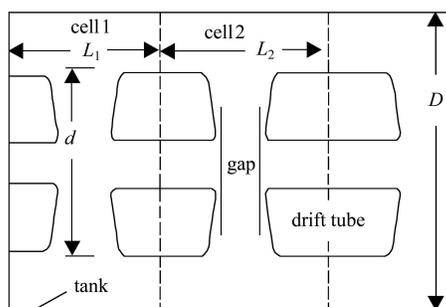
Fig. 1. Schematic diagram of the DTL.
