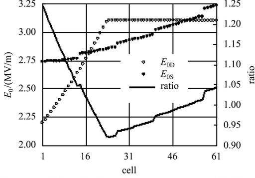
Fig. 2. The  $E_0$  distribution pattern of DTL-1 for CSNS.
