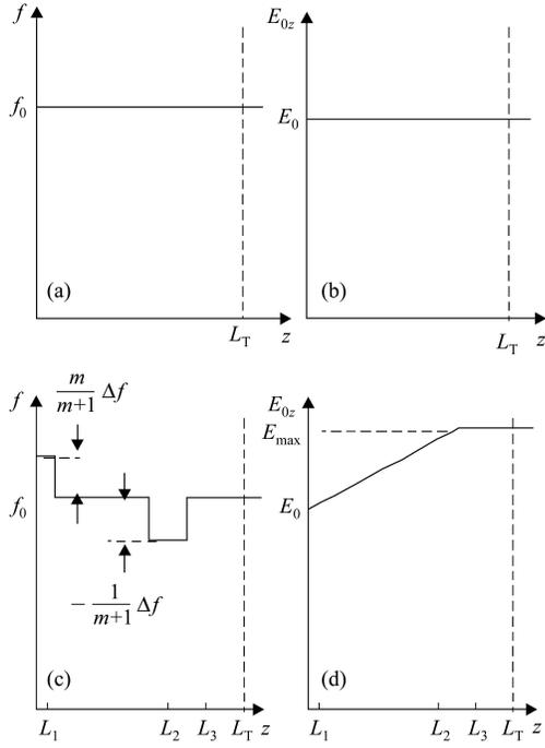
Fig. 3. An example of the effect of local frequency perturbation on a cell chain. (a) Frequency distribution of the unperturbed tank. (b)  $E_0$  distribution pattern of the unperturbed tank. (c) Frequency distribution of the perturbed tank. (d)  $E_0$  distribution pattern of the perturbed tank.
