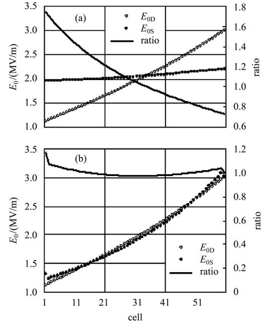
Fig. 6. The  $E_0$  distribution pattern of DTL-1 for SNS. (a) Before tuning. (b) After tuning.
